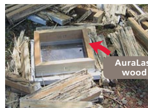
As you can see, after removing the window from its untreated framework, the AuraLast wood clearly withstood the harsh elements of wood decay and termite infestation. AuraLast wood is clearly the survivor!
